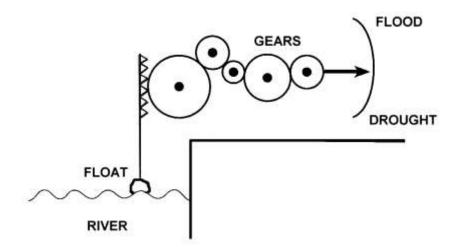
The picture shows a device for registering the level of a river. A float in the river rises and falls and is connected to a gear train. The gear on the right hand side causes a pointer to move up or down.
