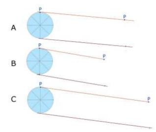
The circumference of the wheel is ∏ times or slightly more than 3 times the diameter of the wheel. If you measure the diameter of the wheel and step it down the ramp, you'll find that A is about right whereas B is clearly too short and C is clearly too long.
