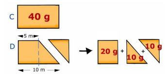
The actual piece removed from shape C and the imaginary second piece are clearly the same shape and size. In other words, they each represent a quarter of shape C's volume (and hence weight). Shape D therefore has three quarters of the weight of shape C or 30g
